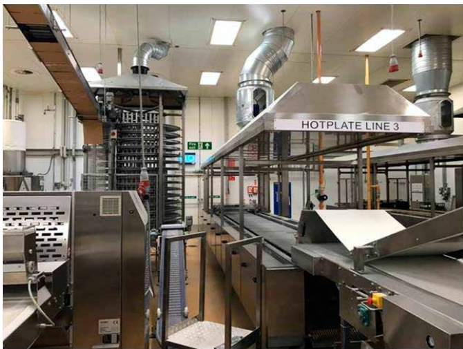
Automatic high output potato scone line
