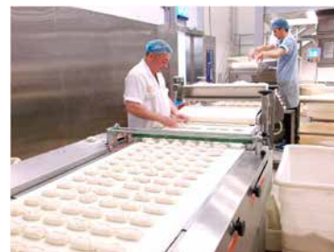
Stress-free cutting line for crispy roll dough pieces
